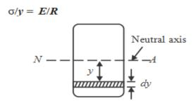
At distance 'y', let us consider an elementary strip of quite small thickness dy. We have already assumed that ' $\sigma$ ' is bending stress in this strip.
