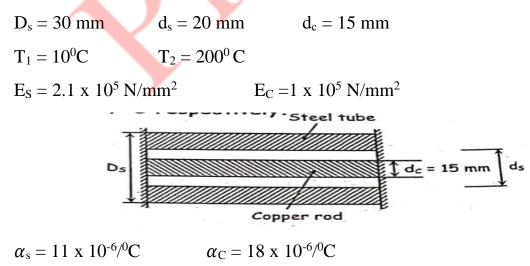
Since  $\alpha_{\rm C} > \alpha_{\rm s}$  compression will be produced in copper and tension in steel.
